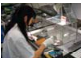
Scattering prevention tray and local exhaust device installed for soldering work
