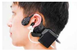
Headset-style wearable system (Image courtesy of TMDU)
